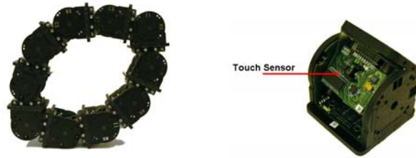
(a) Football shape of a 10 module robot. (b) An individual module.
