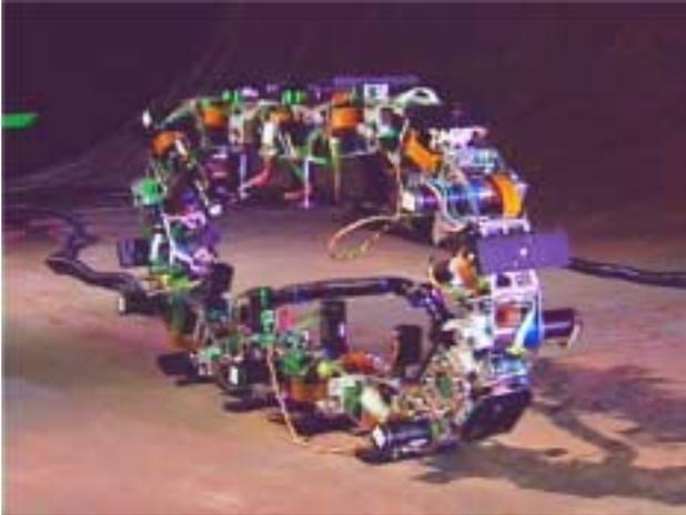
Figure 8: A loop of 23 G2 modules using rolling track locomotion.
