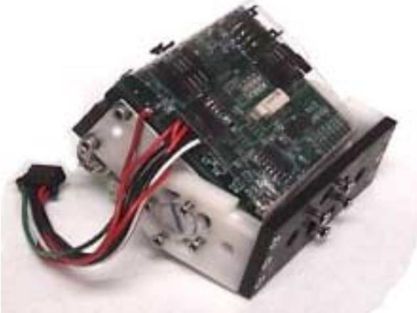
**Figure 2:** A G1v4 module with a communications cable attached. Two of four connection plates are visible. Two AAA batteries are mounted on the backside.
