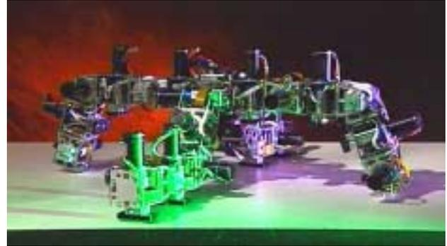
**Figure 11: A four-legged spider-like configuration with G2 modules.**
