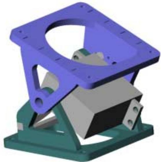
Figure 1: A CAD model of PolyBot G1v3. Modules consist of essentially three parts: two frames and a hobby servo to move them.
