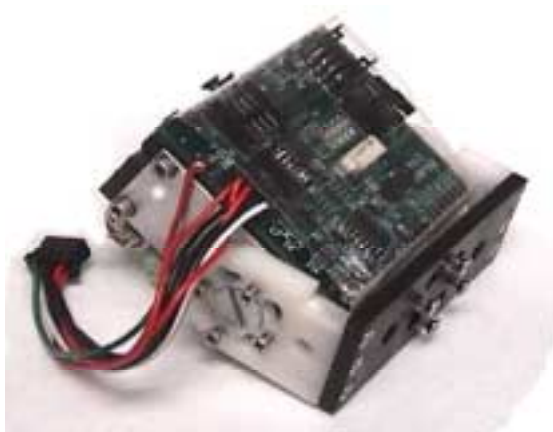
Figure 1: A G1v4 module with a communications cable attached. Two of four connection plates are visible. Two AAA batteries are mounted on the backside.
