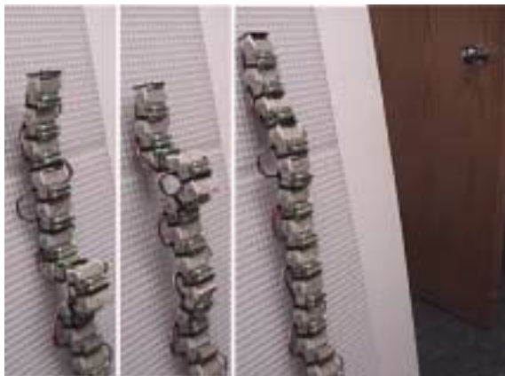
Figure 7: Caterpillar locomotion climbing a near vertical porous material (ceiling tile)
