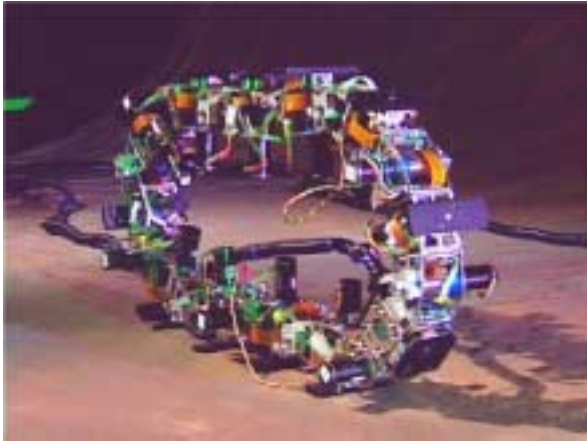
Figure 3: A loop of 23 G2 modules using rolling track locomotion.
