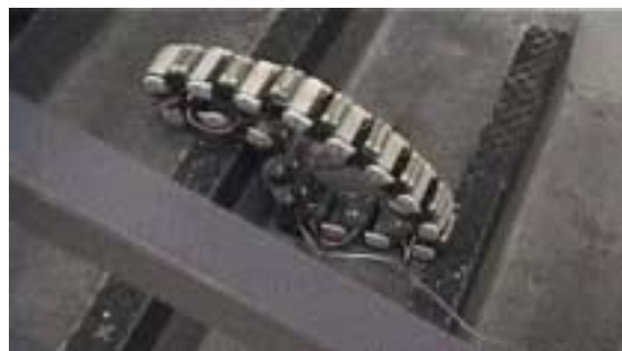
Figure 6: A loop configuration conforming to terrain as it climbs stairs,
