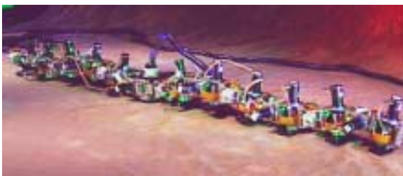
Figure 4: A snake-like sinusoid gait. The travelling wave causes forward locomotion.
