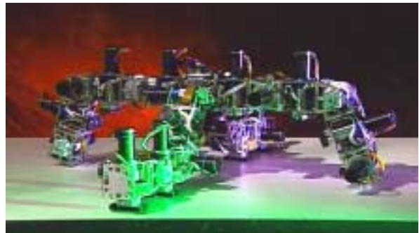
Figure 5: A four-legged spider-like configuration with G1 modules.
