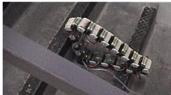
Fig. 10. Stair climbing in the loop form, reaching the next step.
