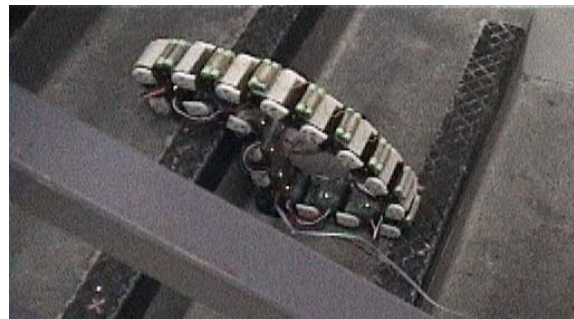
Fig. 11. Stair climbing in the loop form, climbing up the next step.
