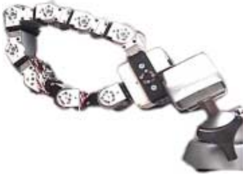
Figure 1: A set of 8 PolyBot G1v4 modules, note the top three are colinear.
