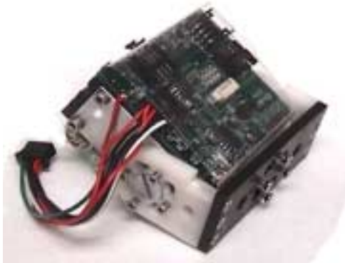
Figure 7: One PolyBot G1v4 module with computer, batteries and one DOF.
